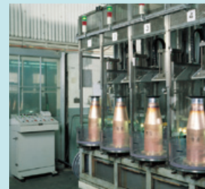
▲ 気密試験装置 Air-tightness testing device
