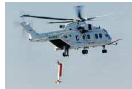
MCH-101に装備する掃海具展張揚収えい航装置 Airborne mine countermeasures stream tow and recovery system
